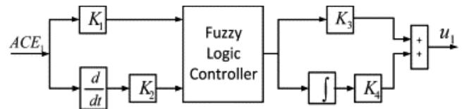
Fig. 2 Structure of model fuzzy PID controller
