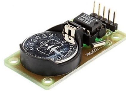
Fig. 3 Module of Real Time Clock DS1302
