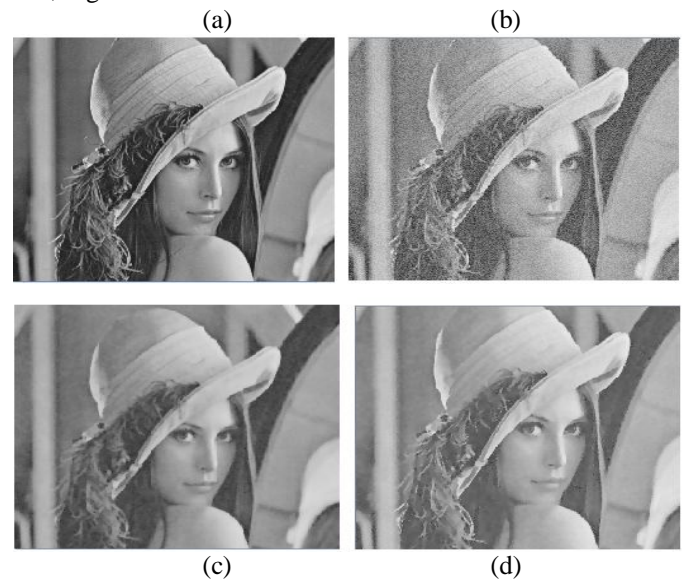
Fig.4.1. Snapshots of output results (a) Original Lena Image, (b) With Gaussian Noise, (c) DEF Image, (d) Fuzzy Filter Image.
