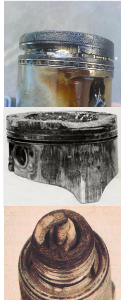
Figure 2.1: Piston & Spark Plug damage due to knocking in Engine
