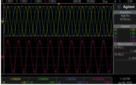
Fig. 4. Output voltage waveforms based SPWM with *R* load
