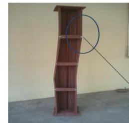
Fig 22 Failure mode of CFS – C – 1 – S – 3
