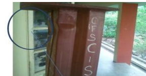
Fig 12. Local Buckling in the web
