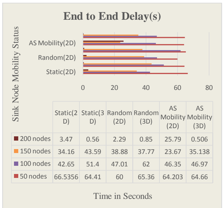
Fig 6: Performance comparison of End to End Delay (Static vs Mobile sink node)
