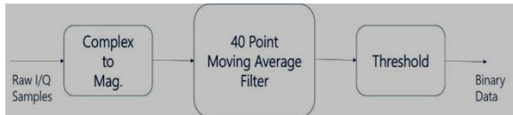
Figure 6: Block Diagram: Signal Decoding
