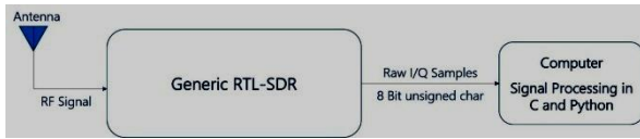
Figure 4: Receiver Block Diagram
