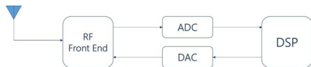
Figure 1: Software Defined Radio Block Diagram
