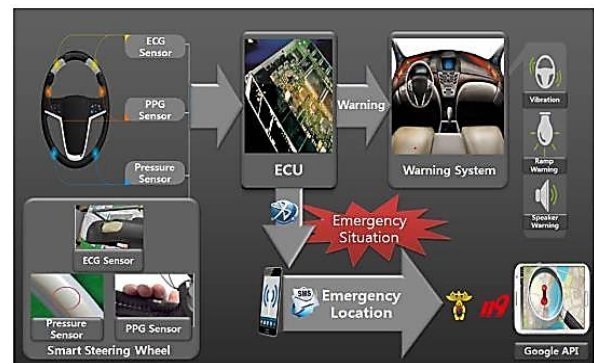
Figure 3. System configuration for smart steering wheel [19]
